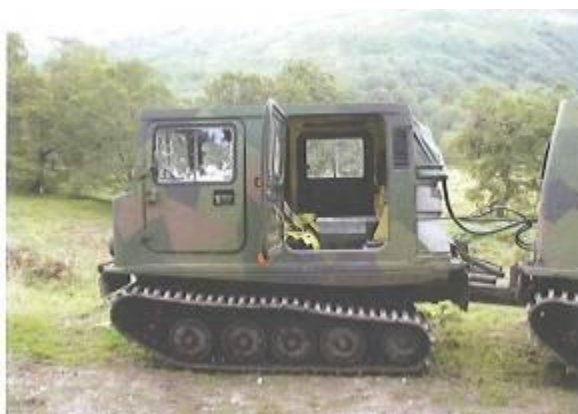
Fig. 17: Example of a personnel carrier in use during wood pole construction (photo included in Environmental Statement, Main Report, pg. 5-9)
